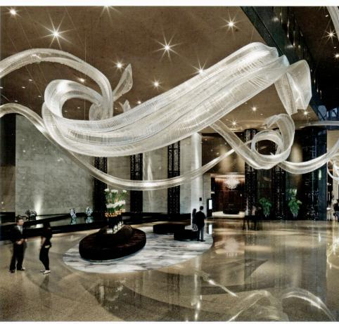
For the 255-foot-long glass ribbon that winds through the lobby of the InterContinental Shanghai Puxi luxury hotel, Weinstein used borosilicate glass tubing with special connectors that allow the finished product to flex and bend. Installed in 2009, it was folded up and placed in a shipping container, and unfurled by a team of 10 after it arrived in China.
